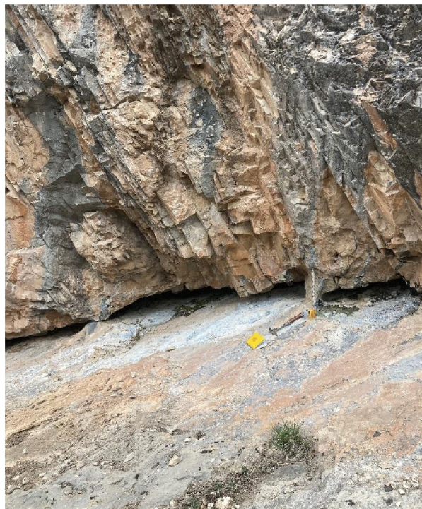
Photo 8: Open aperture of the upper and lower limestone bed where the interbed has been eroded back 3 – 5 feet from the outcrop face. Asperities and direct connections between the two limestone beds creates a rough to very rough surface. (4/14/23 Photo# 2023)
