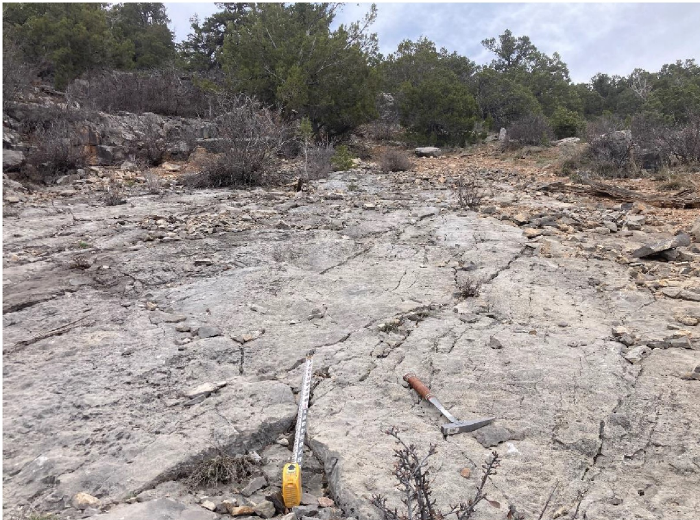
Photo 6: Bedding plane of upper limestone unit exposed within the East drainage. Plane has very high persistence, planar, moderately rough, JRC 10-12. (4/14/23 Photo# 2016)
