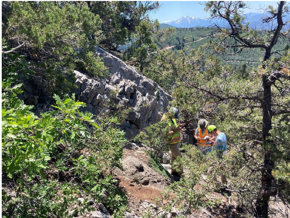
Photo 5: Tape measured 10 ft of lower and upper beds sitting on laterally continuous joint surface. No significant aperture or adverse interbed. Location denoted on Figure 2. (7/6/23 Photo# 2211)
