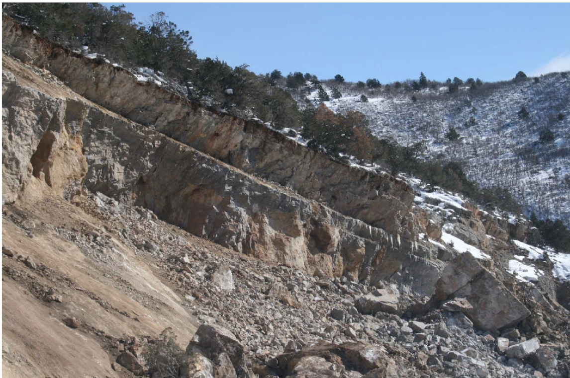
Photo 2: Side view, looking east, of the two upper units of the limestone with bedding acting as the slide plane. The upper limestone units pinch out upslope, to the north (1/26/23 Photo# 0598)
